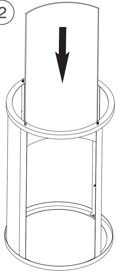
1. Assemble all 4 metal dividers to the top and bottom rings. Start at the bottom, then add the top ring.
